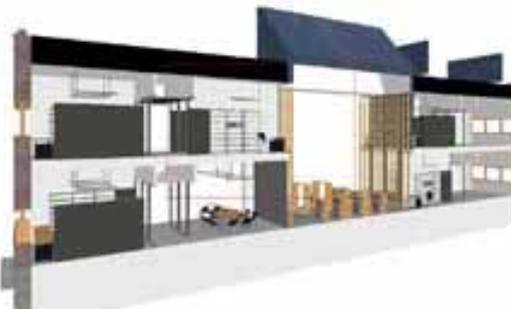
A shared building information model was developed at the outset, at the request of Senate Properties. The architect and contractor were required to work with the model, which was IFC-based.
